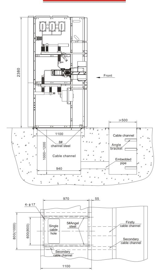
KGN $\square$ -12 Fixed type switchgear sketch of foundation installation
